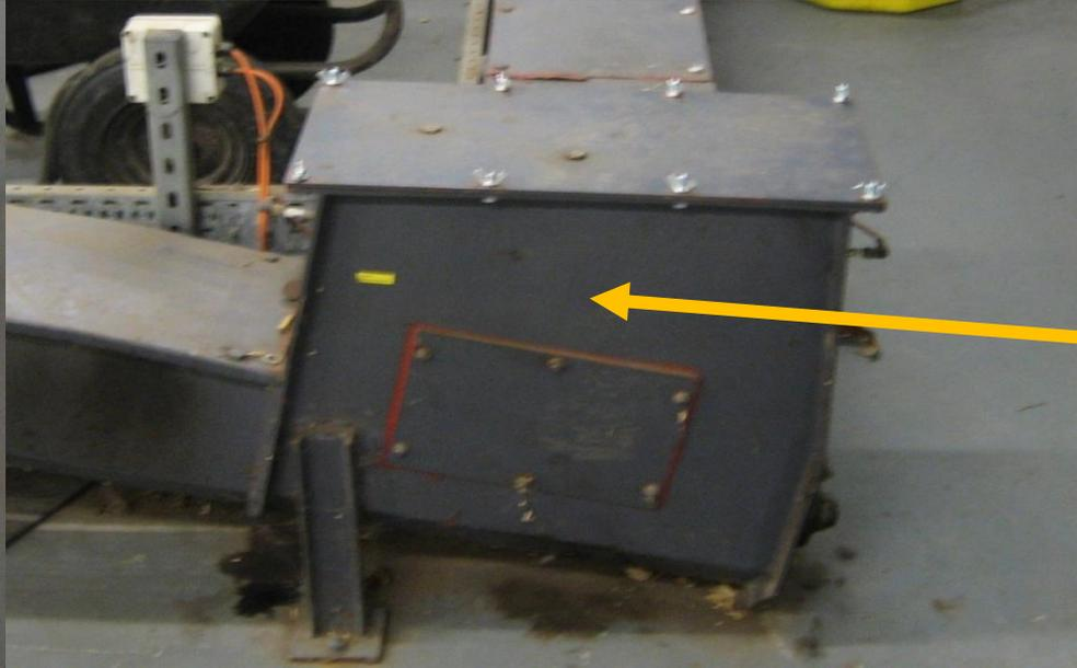
Metering bin fuel blockage point when oversize wood chips are present in the fuel supply
