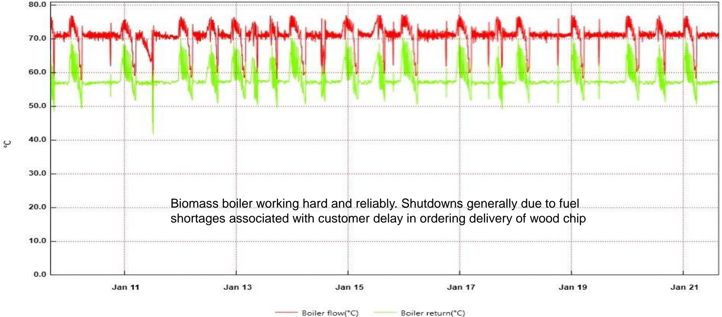
Biomass boiler working hard and reliably. Shutdowns generally due to fuel shortages associated with customer delay in ordering delivery of wood chip
