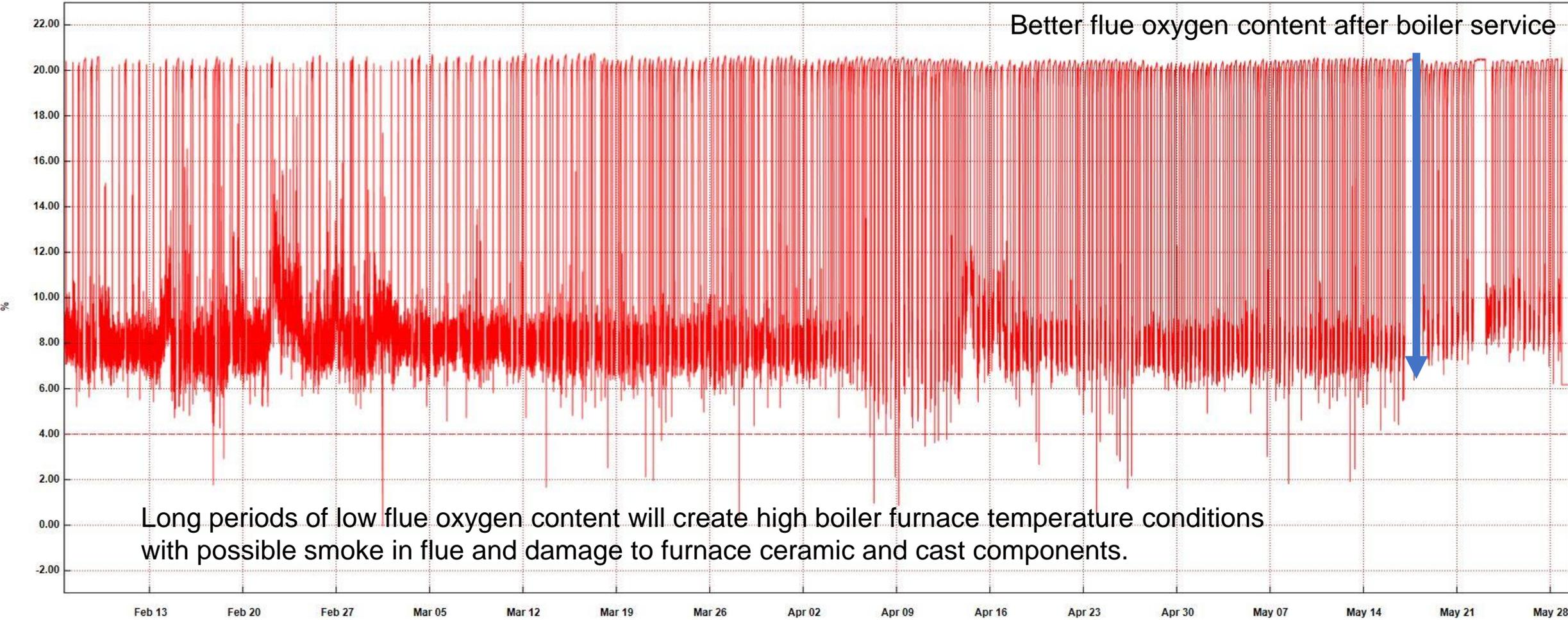
Long periods of low flue oxygen content will create high boiler furnace temperature conditions with possible smoke in flue and damage to furnace ceramic and cast components.
