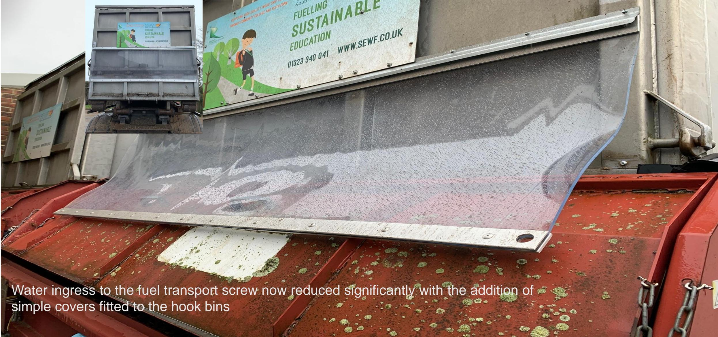
Water ingress to the fuel transport screw now reduced significantly with the addition of simple covers fitted to the hook bins
