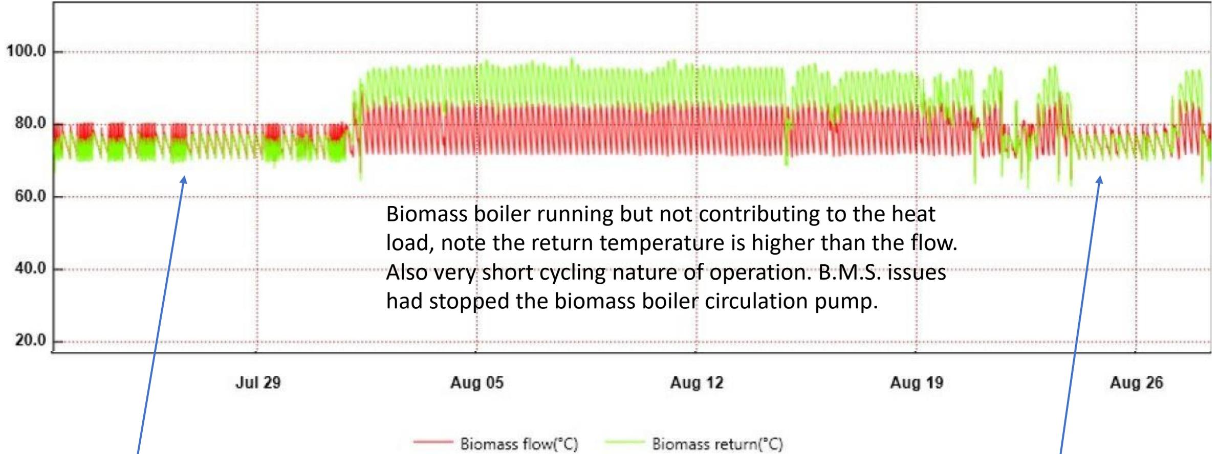
Biomass boiler running but not contributing to the heat load, note the return temperature is higher than the flow. Also very short cycling nature of operation. B.M.S. issues had stopped the biomass boiler circulation pump.
