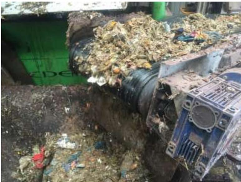
Photo 4. Removed packaging after washing before being pressed
